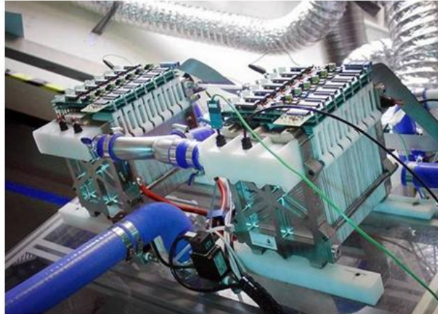
25kW PEM Fuel Cell
